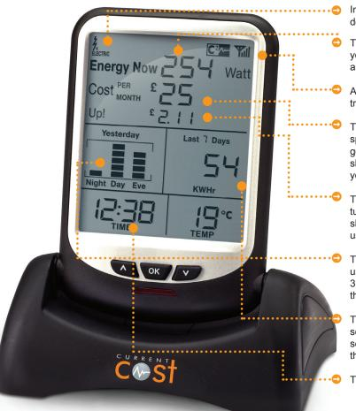
Indicates the number of sensor jaws installed. For most domestic situations this will be one
